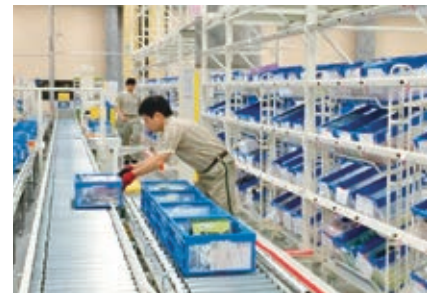
FRAPS,* installed in parallel inside a TA-Q-BIN terminal * FRAPS is an acronym for the Free Rack Auto Pick System, a cloud-based setup that can use "last mile" networks. This picking system uses proprietary flow-through racks.
