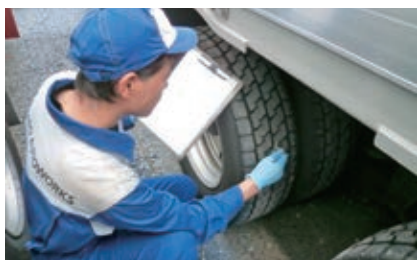
Checks include tire tread depth and air pressure
